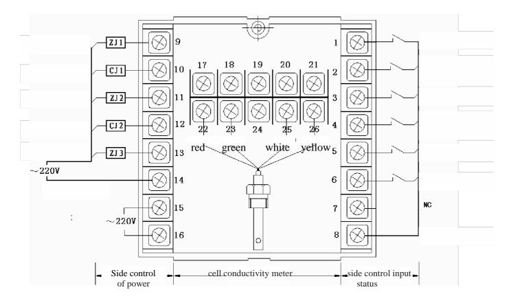
Attention: The controller is working with low-power relays, using large inductive load must be applied with relays or contactors. Direct connection will damage the contact or shorten its life.
